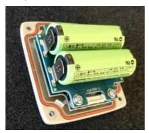
• Place the front panel and fix it with the 4 screws.
