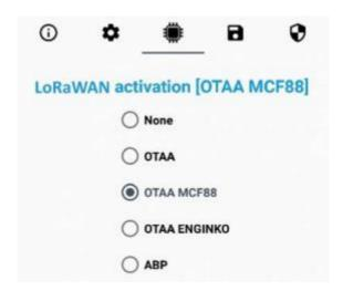
The device exits factory activated with **NONE** mode. On request devices can be shipped already activated. Note: in **OTAA** AppKey is write only, in reading the field will always be empty, even if set.
