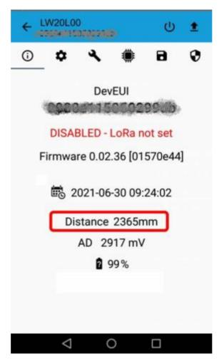
Once provisioned on a LoRaWAN® network, the device sends the distance & timestamp to the server via uplink.
