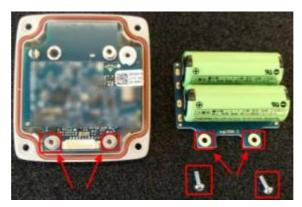
• Place the new PCB batteries pack and put them in place with the screws:
